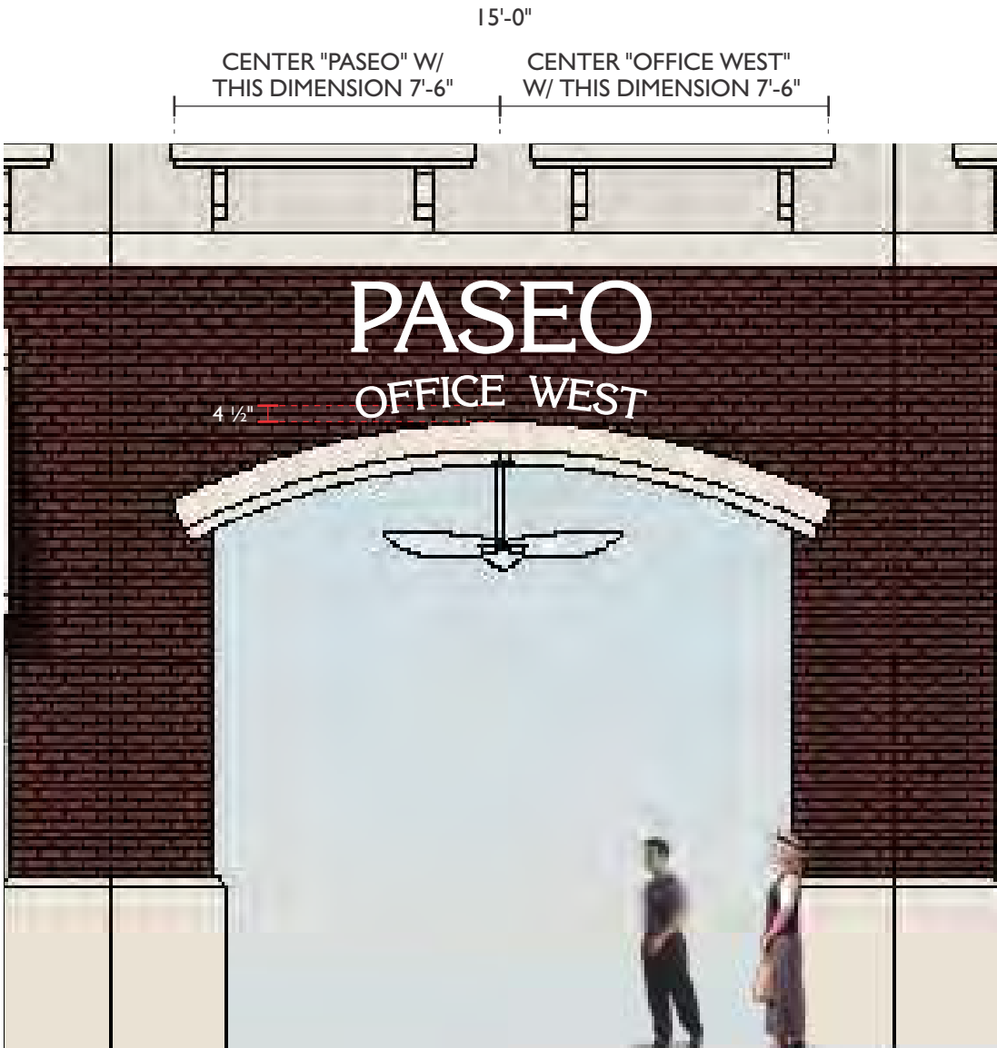
BUILDING "K" EAST ELEVATION DETAIL 1/4" = 1'
