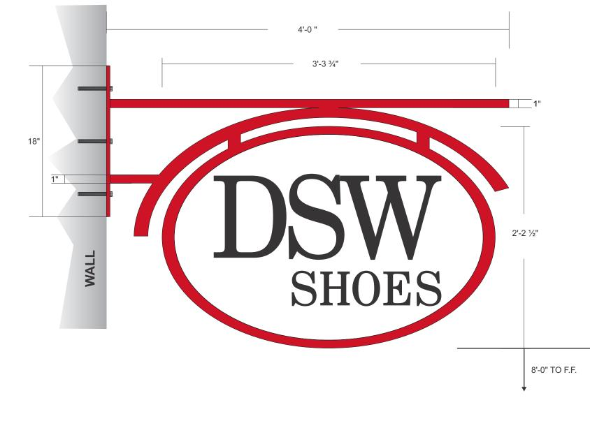
SIGN SUPPORTS 1" x 2" SQ. TUBE ALUM. W/ A-18" x 5" PLAQUE FLUSH MOUNTED TO WALL, PTD PER TENANT LAYOUT.
